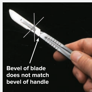
Figure 1.7 Scalpel Blade Placement. (a) Correct procedure. (b) Incorrect placement of a blade on a blade handle. Notice that the bevel on the blade does not match up with the bevel on the blade handle. If placed in this fashion, the blade will not be secure on the handle and may slip off the handle and injure someone.
