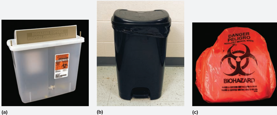
Figure 1.4 Common Laboratory Waste Receptacles. (a) Sharps container. (b) Waste basket. (c) Hazardous waste bag.
